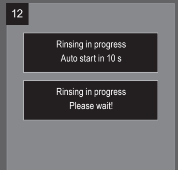
Automatic external rinsing: 5 min after the last milk-based beverage preparation an automatic rinsing of the milk system for approx. 25 s is started.
